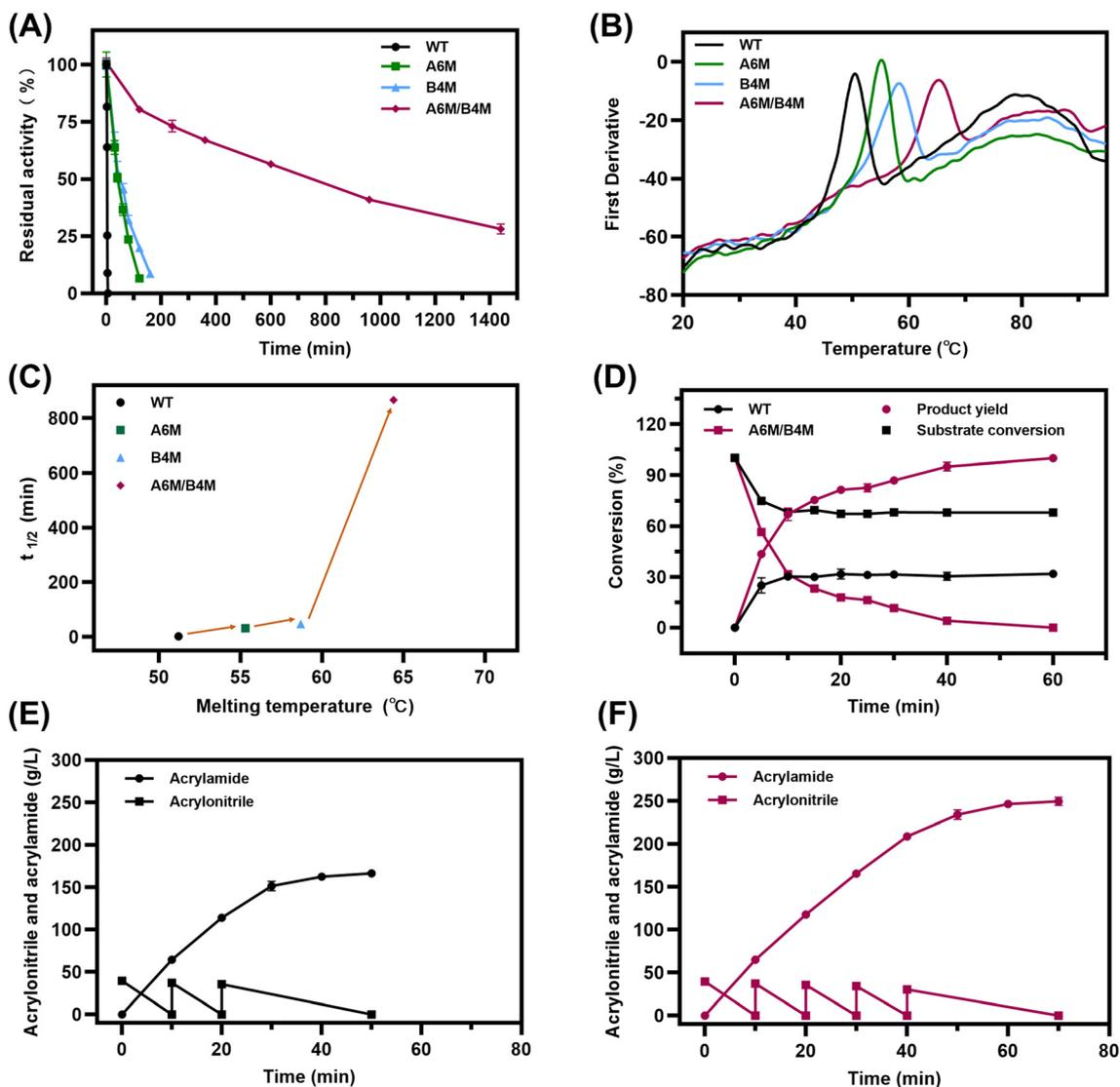
Fig. 4 (A) Deactivation curve at 50 °C. (B) Curves of thermal denaturation. (C) Enhancing the thermostability of A6M/B4M by integration of two subunits presented by both kinetic and thermodynamic stability. (D) Catalytic reaction process catalyzed by WT and A6M/B4M. (E) Fed-batch reaction for the synthesis of acrylamide using WT. (F) Fed-batch reaction for the synthesis of acrylamide using A6M/B4M.
