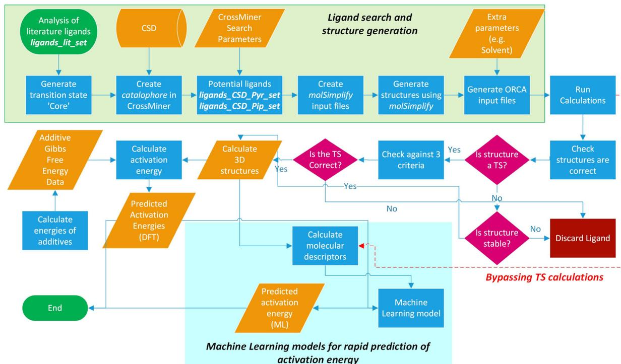
Fig. 2 Workflow overview for identifying ligands in the CSD, high-throughput calculation of  $\Delta G^\ddagger$ , and ML prediction of  $\Delta G^\ddagger$  for *in silico* screening of catalysts.
