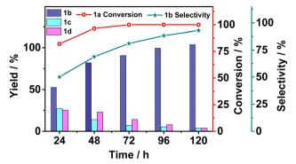
Fig. 2 The product yields from photocatalytic  $C_{\alpha}$ – $C_{\beta}$  bond cleavage of **1a** over the elapsed time. 1b selectivity = moles of product 1b/moles of product (1b + 1c + 1d)  $\times$  100%.
