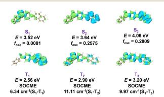
Fig. 3 Iso-surface maps of the electron-hole density difference of  $\mathbf{6}$ 's  $S_n$ and  $T_n$  states calculated in Gaussian 16 by TD-DFT/B3LYP/6-31G(d,p), where blue and green iso-surfaces correspond to hole and electron distributions, respectively, and SOCME values calculated on ORCA 4.2.1 by TD-DFT/B3LYP/def2-TZVP(-f).
