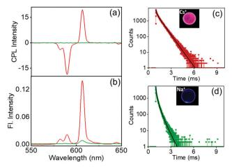
Fig. 4 (a) CPL and (b) fluorescence spectra of  $Cs^{+}[Eu((+)-tfac)_{4}]^{-}$  (red traces) and Na<sup>+</sup>[Eu((+)-tfac)<sub>4</sub>]<sup>-</sup> (green traces) embedded in the PMMA films. (c and d) Luminescence lifetime plots of the hybrid PPMA films composed of (c)  $Cs^{+}[Eu((+)-tfac)_{4}]^{-}$  and (d)  $Na^{+}[Eu((+)-tfac)_{4}]^{-}$  ( $\lambda_{ex}$  = 352 nm). The inset shows the photographs of the corresponding films collected upon excitation using a 365 nm UV lamp.
