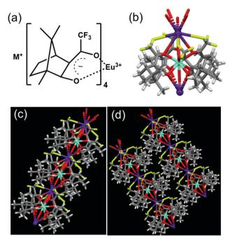
Fig. 2 (a) Molecular structure of  $M^{+}[Eu((+)-tfac)_{4}]^{-}$  (M = Na, K, Rb, Cs). (b-d) X-ray crystal structure of (b) the  $Cs^+[Eu((+)-tfac)_4]^-$  complex, (c) its one-dimensional array and (d) the network structures.
