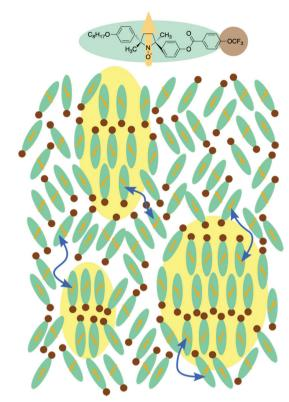
Fig. 7 Molecular orientations in and out of the cybotactic clusters. Molecules of  $(\pm)$ -3 have the trifluoromethyl group (brown circles) and electron spins of nitroxide radical moieties (orange arrows). The molecules move into and out of the yellow-colored cybotactic clusters. Blue doubleheaded arrows denote the molecular exchange inside and outside the cybotactic clusters
