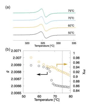
Fig. 6 EPR spectroscopy of  $(\pm)$ -3 upon the cooling run. Black and orange circles denote the g-value and  $\chi_{\text{rel}}$  respectively. Vertical dotted line denotes the N-to-N<sub>cyb</sub> phase transition point.
