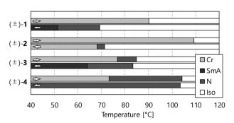
Fig. 4 Phase transition behaviors of compounds  $(\pm)$ -1-4. DSC analyses determined transition temperatures at a scanning rate of 5 °C min<sup>-1</sup> upon the heating and cooling run.
