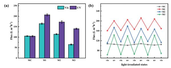
Fig. 7 Photo-responsive performances of PRMs: (a) pure water flux of MC, M1, M2 and M3 for irradiation of visible and UV light; (b) pure water flux of MC, M1, M2 and M3 when the irradiation light was switched for four cycles.
