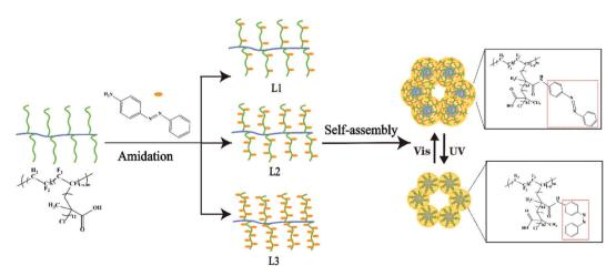
Fig. 1 Schematic of the functional polymer preparation and the photo-responsive function.
