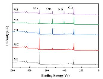
Fig. 4 XPS wide scans of the prepared membranes.
