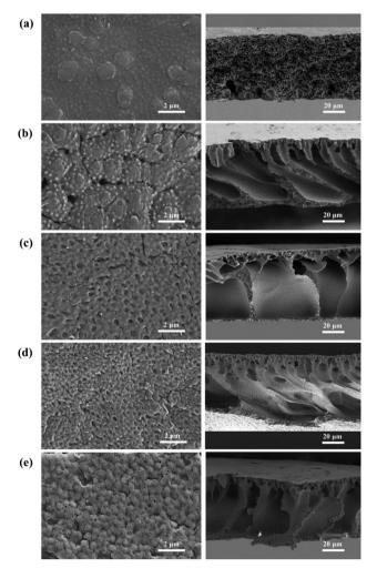
Fig. 5 SEM images of the surfaces (left) and the cross-sections (right) of (a) M0, (b) MC, (c) M1, (d) M2 and (e) M3
