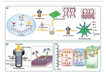
Scheme 1 (a) Synthesis diagrams of Mo modified InOOH/In(OH)<sub>3</sub>. (b) Schematic diagram of the  $CO_2$  photo-reaction system. (c) The proposed mechanism diagram of photocatalysis under visible-light irradiation ( $\lambda$  > 420 nm).
