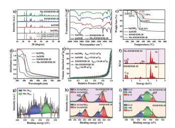
Fig. 2 (a) XRD patterns, (b) FT-IR spectra, (c) TGA curves, (d) UV-vis diffuse reflectance spectra, and (e)  $\rm N_2$  adsorption–desorption isotherms of  $\rm In(OH)_3$ ,  $\rm InOOH, IOOH/IOH-20$ , and  $\rm Mo-IOOH/IOH-20$ . (f) EDS spectra of  $\rm IOOH/IOH-20$  and  $\rm Mo-IOOH/IOH-20$ . (g) XPS spectrum for  $\rm Mo-IOOH/IOH-20$  in the region of Mo 3d. (h and i) XPS spectra for  $\rm IOOH/IOH-20$  and  $\rm Mo-IOOH/IOH-20$  in regions of In 3d and O 1s.
