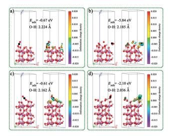
Fig. 7 CO<sub>2</sub> adsorbed on the (001) surface of In(OH)<sub>3</sub> with different section thicknesses, exposed atoms, and adsorption sites: (a)  $In_8CO_{26}H_{24}$ , (b)  $In_8CO_{30}H_{28}$ , (c)  $In_{12}CO_{38}H_{36}$ , and (d)  $In_{12}CO_{40}H_{40}$ .
