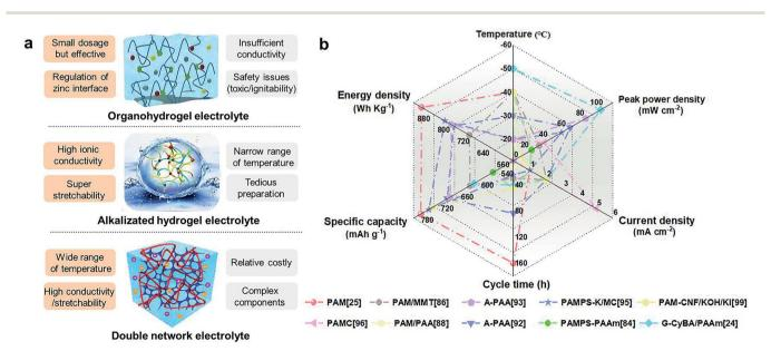
Fig. 11 (a) The comparison of the three design strategies for low-temperature resistant GPEs. Orange for pros and grey for cons. Reproduced with permission from ref. 92. Copyright 2020, Wiley. Reproduced with permission from ref. 24. Copyright 2021, Elsevier. (b) The performance of previously reported ZABs with low-temperature resistant hydrogels.
