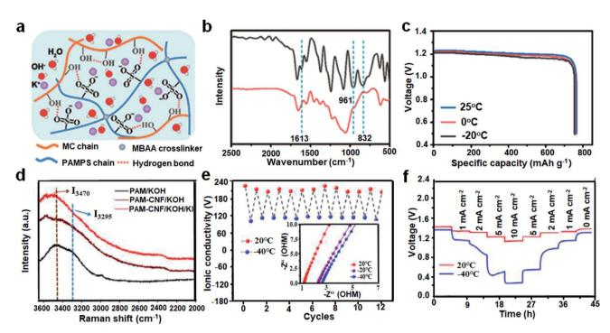
Fig. 10 (a) Schematic diagram of the PAMPS-K/MC hydrogels. (b) FT-IR spectra of the freeze-dried PAMPS/MC hydrogels (red) and the mixture of AMPS/MC (black). (c) Specific capacity of the ZABs at different temperatures. Reproduced with permission from ref. 97. Copyright 2021, American Chemical Society. (d) Raman spectra. (e) Ionic conductivity at 20 and  $-40\,^{\circ}$ C. (f) Rate performance. Reproduced with permission from ref. 101. Copyright 2021, Elsevier.
