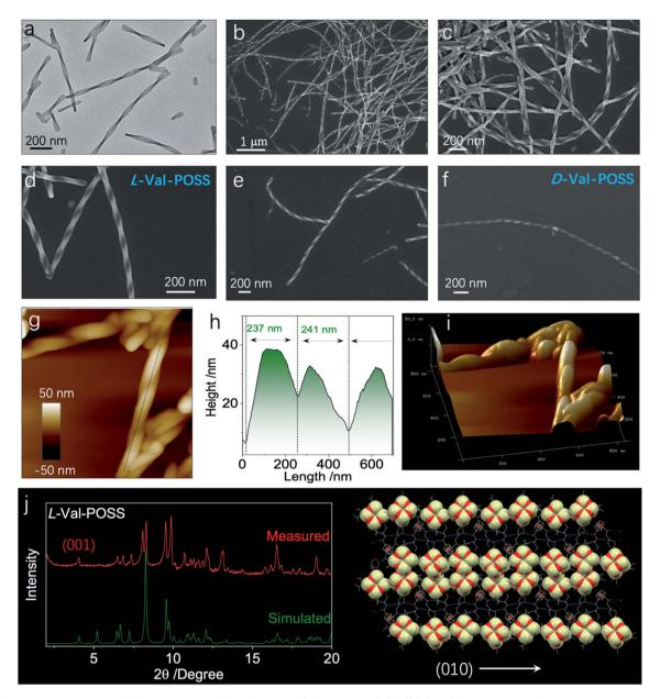
Fig. 5 (a) TEM image of L-Val-POSS self-assembly (1 mM) in a THF/ACN mixture (1/9, v/v). (b-e) Corresponding SEM images of L-Val-POSS selfassembly at different magnifications. (f) SEM image of D-Val-POSS under the same conditions. (g and h) AFM (840 × 840 nm) and height profile of Val-POSS self-assembly. (i) Corresponding 3D AFM image. (j) Powder XRD pattern comparison as well as the speculated 1D growth of Val-POSS directed by hydrogen bonds.
