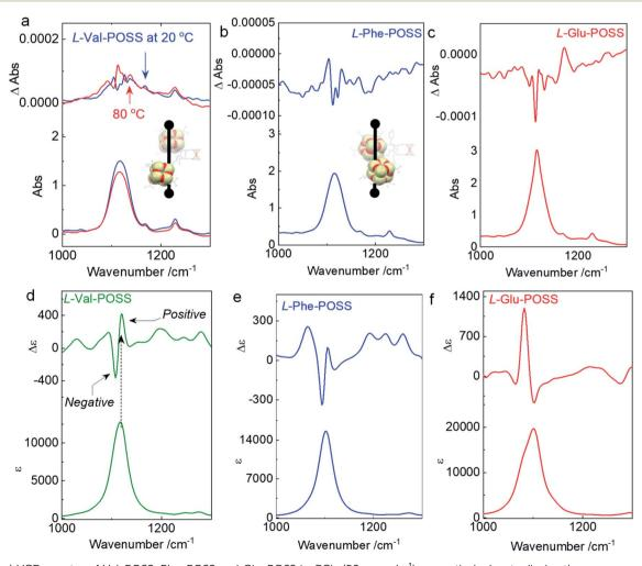
Fig. 4 (a-c) VCD spectra of Val-POSS, Phe-POSS and Glu-POSS in CCl<sub>4</sub> (50 mg mL<sup>-1</sup>) respectively. Insets display the corresponding intramolecular folding of POSS segments. (d-f) Calculated VCD spectra of Val-POSS, Phe-POSS and Glu-POSS respectively via time-dependent DFT (TDDFT) at B3LYP/6-31g(d) level of theory (full width at half maximum =  $15 \text{ cm}^{-1}$ ).
