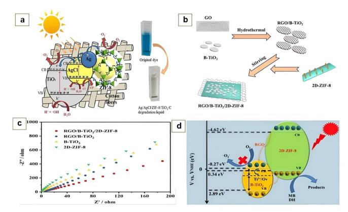
Fig. 6 (a) Photo-degradation mechanism of MB with Ag/AgCl/ZIF-8/TiO $_2$ /C hybrid. Reproduced from ref. 126 Copyright 2019, Springer. (b) Process for the elaboration of the ternary system RGO/B TiO $_2$ /2D-ZIF-8. (c) EIS analysis of B-TiO $_2$ , RGO/B TiO $_2$ , 2D-ZIF-8 and RGO/B TiO $_2$ /2D-ZIF-8. (d) Photo-degradation mechanism of MB with RGO/B TiO $_2$ /2D-ZIF-8 ternary system. Reproduced with permission from ref. 127 Copyright ©2020, Wiley VCH.
