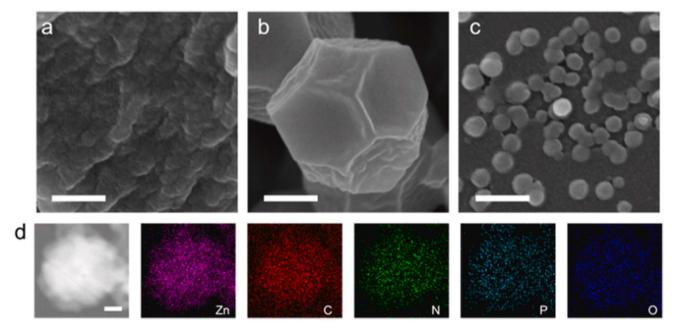
Fig. 2 SEM images of ZnAMP (a), ZIF-8 (b) and NZIF (c) (scale bar is 200 nm). (d) HAADF image of NZIF and EDS mapping of Zn, C, N, P and O, where P and O are exclusive to the nucleotide (scale bar is 20 nm). Reproduced with permission from ref. 78 Copyright ©2021, Elsevier.
