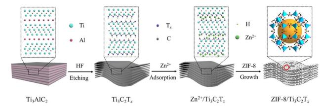
Fig. 3 Illustration of the synthesis of ZIF-8/Ti<sub>3</sub>C<sub>2</sub>T<sub>x</sub>. Reproduced with permission from ref. 86 Copyright ©2022, Elsevier.
