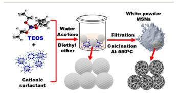
Fig. 3 Preparation of mesoporous silica as nanoporous carrier. Briefly, TEOS (tetraethoxysilane) is reacted with a cationic surfactant (e.g., CTAB) in water/acetone/diethyl ether solvent to form mesoporous silica nanospheres (MSNs). Filtration is then carried out followed by calcination at 550 °C.
