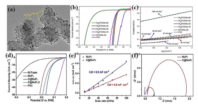
Fig. 14  $Ni_2P$  supported on carbon nanospheres: (a) TEM image, (b) LSV curves in 0.5 M  $H_2SO_4$  and (c) corresponding Tafel plots (reproduced from ref. 78 with permission from Elsevier, Copyright 2015). Carbon-coated  $Ni_8P_3$ : (d) LSV curves in 0.5 M  $H_2SO_4$ , (e) electrochemical double-layer capacitance and (f) EIS plots (reproduced from ref. 108 with permission from the America Chemistry Society, Copyright 2016).
