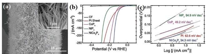
Fig. 12 NiCo<sub>2</sub> $P_x$  nanowire arrays: (a) SEM image, (b) LSV curves in 1.0 M KOH and (c) corresponding Tafel plots (reproduced from ref. 111 with permission from Wiley, Copyright 2017).
