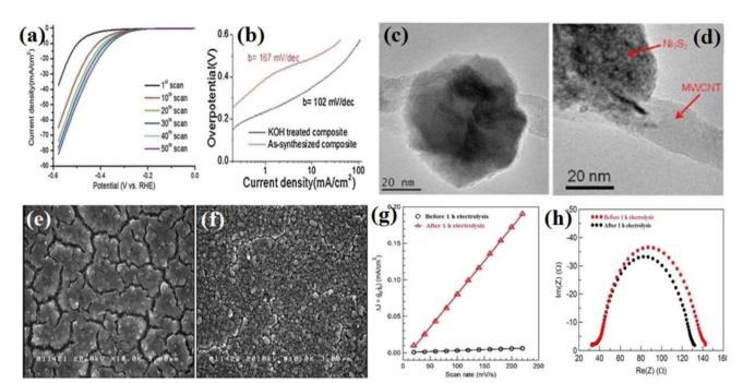
Fig. 9  $N_{13}S_{2}(55\%)/MWCNT-NC$ : (a) LSV curves at different polarization values in 30 wt% KOH and (b) corresponding Tafel plots before and after 12 h base treatment in 30 wt% KOH. (c) TEM image before base treatment and (d) TEM image after base treatment (reproduced from ref. 101 with permission from Elsevier, Copyright 2014). Ni–S/FTO: (e) SEM image before 1 h electrolysis, (f) SEM image after 1 h electrolysis, (g) electrochemical double-layer capacitance and (h) EIS plots.
