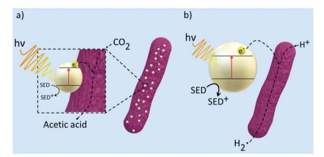
Fig. 5 General mechanism for electron transfer between a semiconductor and microbe in a hybrid photosystem. (a) Direct photoreduction of  $CO_2$  to acetic acid in which the semiconductor is deposited onto the surface of the microbe (b) indirect photoreduction of  $CO_2$  to  $H_2$  by colloidal nanoparticles in the presence of electron mediators and SEDs.
