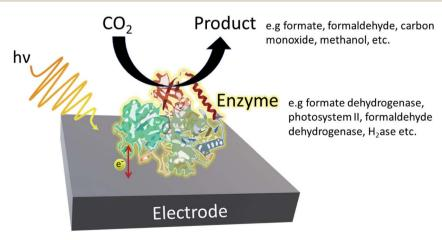
Fig. 3 Example of a typical enzymatic photohybrid system in which CO<sub>2</sub> is reduced by the enzyme to produce the appropriate biofuel.
