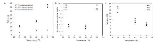
Fig. 9 (a) Dimensions of BCS ellipsoidal aggregates with variation of  $M_n$  and temperature, derived from SANS fitting, (b) ratio of equatorial to polar radii, and (c) degree of hydration of BCS particles estimated from the values of the SLDs returned by the fits. The parameters for P6 are omitted due to the different approach to fitting used and the presence of multiple species in solution.
