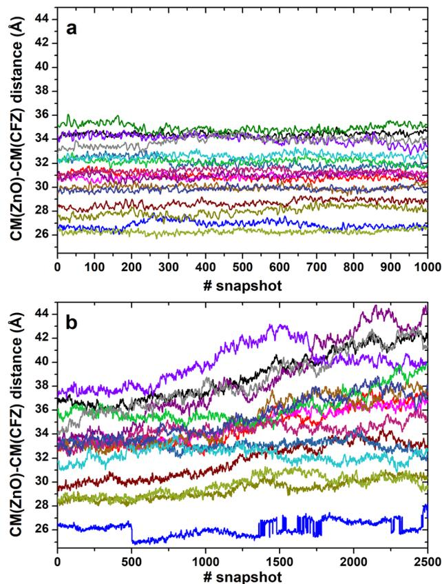
**Fig. 8** Evolution of the distance between the center of mass of the ZnONP and the center of mass of each adsorbed CFZ molecule (represented by the various color lines) in ethanol (last 200 ps) (a) and water (last 500 ps) (b) solutions.
