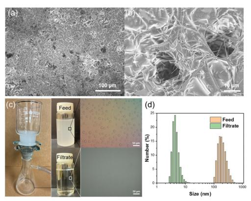
Fig. 5 (a) and (b) SEM images of a T-ZnO/PLMA coated quantitative filter paper. (c) Photographic and optical microscopy images of a surfactantstabilized water-in-hexane emulsion before and after being filtered through the T-ZnO/PLMA coated filter paper. (d) Normalized water size distribution of the feed and filtrate measured by dynamic light scattering.
