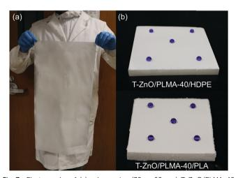
Fig. 7 Photographs of (a) a large size (30  $\times$  60 cm) T-ZnO/PLMA-40 coated mesh; and (b) T-ZnO/PLMA-40 coated HDPE and PLA sheets with dyed blue water droplets.
