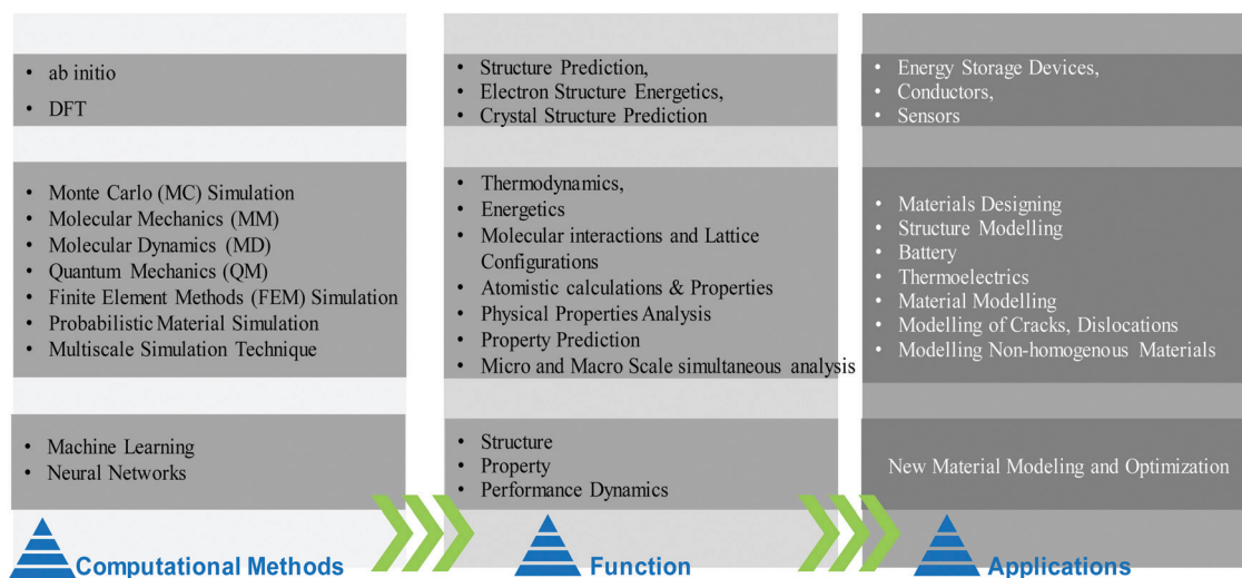
Fig. 7 Various computational methods involved in materials modeling, simulation, and property prediction. Quantum mechanical methods like ab initio and DFT are widely used for structure prediction and calculating interatomic interactions and have been applied in the development of energy devices and sensors. Similarly, various simulation techniques have roles in atomistic, energetic calculations and are applied for new materials designing and modeling of non-homogenous materials. Big Data analysis approaches like ML and NN are used to train and predict materials structure and properties using data from various databases.
