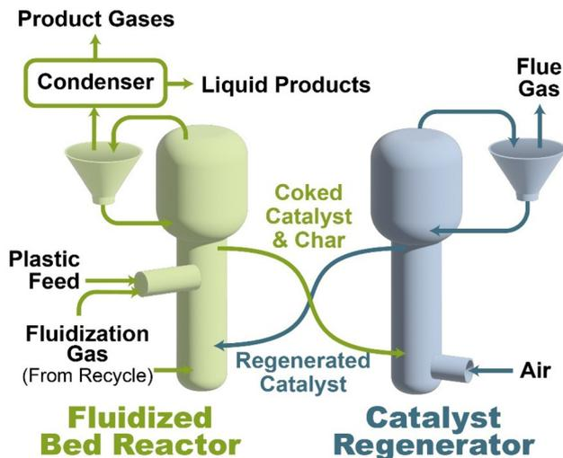
Fig. 22 Fluidized bed reactor for plastic pyrolysis.<sup>508</sup>
