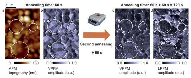
Fig. 4 Ferroelectric domains before and after a second annealing step. (a) Sample topography. (b) The VPFM amplitude of a sample after the initial 60 s of annealing shows out-of-plane polarized domains. (c) After the second annealing for 60 s, the vertical domains shrink in size and partly vanish (marked in white). (d) At the same time, alternating domains with in-plane polarization occur in LPFM, displacing the vertical domains.
