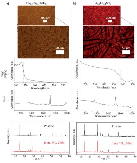
Fig. 5 Optical image, absorption spectra, FTIR spectra and XRD pattern for (a) FA<sub>0.9</sub>Cs<sub>0.1</sub>PbBr<sub>3</sub> and (b) FA<sub>0.9</sub>Cs<sub>0.1</sub>SnI<sub>3</sub> perovskite thin films, annealed at 1.4 s  $t_{\rm f}$
