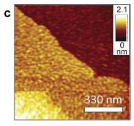
Fig. 1 (a) X-ray diffractogram of a 20 nm LaNiO<sub>3</sub> film on Nb:SrTiO<sub>3</sub>. The (002) substrate peak is marked with a star, the (002)  $_{10}$  film peak with an arrow. (b and c) Atomic force microscopy (AFM) of a 20 nm LaNiO<sub>3</sub> film with different magnification. AFM was performed after UHV transfer from the deposition tool to the analysis chamber.
