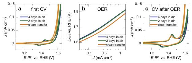
Fig. 3 (a) First sweep during cyclic voltammetry in the Ni redox region with representative 20 nm LaNiO<sub>3</sub> thin film electrocatalysts. (b) Cyclic voltammetry in the OER potential regime. The average between anodic and cathodic sweep of the second cycle is shown. (c) First sweep during cyclic voltammetry in the Ni redox region after two sweeps to OER potentials. Scan rate was 10 mV s<sup>-1</sup> for all panels.
