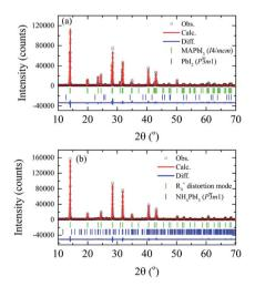
Fig. 4 X-ray powder diffraction data and Rietveld refinements at room temperature of the (a) MAPbl $_3$  as-compacted sample and (b) submitted to thermal annealing at 250 °C for 40 hours.
