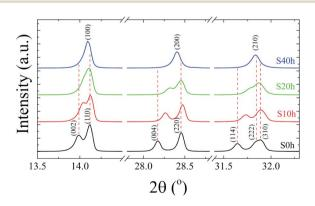
Fig. 2 Room-temperature X-ray diffraction patterns of the pelletized MAPbl<sub>3</sub> sample after being submitted to a heat treatment at  $T = 250 \,^{\circ}\text{C}$ for different annealing times, t = 0, 10, 20, and 40 h.
