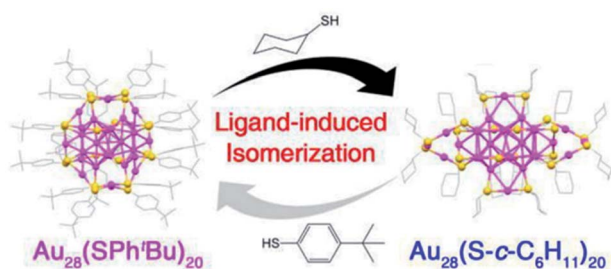
Fig. 15 Ligand-exchange induced transformation between \text{Au}_{28}(\text{SPh}^t\text{Bu})_{20} and \text{Au}_{28}(\text{S}-c\text{-C}_6\text{H}_{11})_{20} nanoclusters. Color codes: purple sphere, Au; yellow sphere, S; gray sphere, C. For clarity, all H atoms are omitted. Adapted with permission from ref. 59. Copyright 2016 American Chemistry Society.
