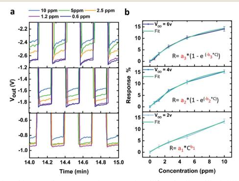
Fig. 3 (a) Output voltage of the inverter after exposure to various concentrations of NO<sub>2</sub> gas for a  $V_{in}$  at -4 V and -11 V alternatively for three different  $V_{DD}$  values (from top to bottom:  $V_{DD} = 6$  V, 4 V and 2 V). (b) Response of the inverter as a function of NO<sub>2</sub> concentration for the three different  $V_{DD}$  values (from top to bottom:  $V_{DD} = 6$  V, 4 V and 2 V).
