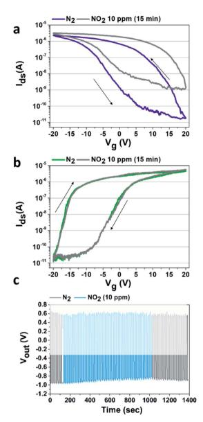
Fig. 2 (a)  $I_{ds}-V_g$  characteristic of the p-type SWCNT-FET before and after 15 min of NO<sub>2</sub> exposure ( $V_{DS} = 1$  V). (b)  $I_{ds}-V_g$  characteristic of the n-type SWCNT-FET before and after 15 min of NO<sub>2</sub> exposure ( $V_{DS} = -1$  V). (c) Output voltage as a function of time of the inverter under an exposure of NO<sub>2</sub> gas for a square input voltage for alternatively -4 V and -11 V ( $V_{DD} = 2$  V).
