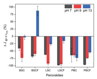
Fig. 3 Results of potential stability tests, where the changes of current density are plotted after 500 cycles of potential steps from 1.0 to 1.6  $V_{RHF}$ holding each potential for 10 seconds. This measurement was carried out in electrolytes of pH 7, 9, and 13.
