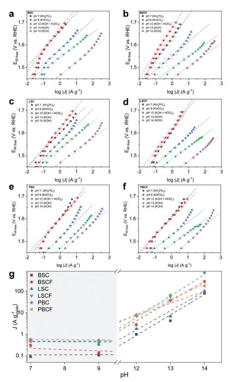
Fig. 2 Tafel plots are constructed from series of chronoamperometry measurements comparing OER activities at different pH levels for each prepared catalyst (a–f). Markers represent the current densities at 1.58 V<sub>RHE</sub> of the studied perovskites in logarithmic scale with respect to pH depicting the order of activity (g).
