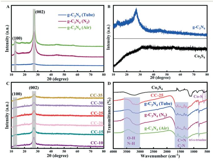
Fig. 1 XRD patterns of (A)  $g-C_3N_4$  (prepared using different methods), (B)  $Co_3S_4$  and  $g-C_3N_4$  tube, (C) CC-x (x = 10, 15, 20, 25, 30, 35), and (D) FT-IR spectra of g-C<sub>3</sub>N<sub>4</sub> (prepared using different methods), Co<sub>3</sub>S<sub>4</sub>, and CC-25.
