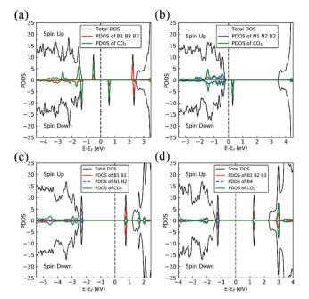
Fig. 14 Spin-polarized total density of states (TDOS) (black line), and spinpolarized PDOS of defect area (red line or blue line) and of adsorbed CO2 (green line) of  $CO_2$ -dh-BN with (a)  $V_N$ , (b)  $V_B$ , (c) SW, and (d)  $B_N$ , respectively. The position of the Fermi level ( $E_F$ ) is indicated by dashed line.
