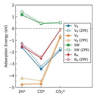
Fig. 19 Adsorption energy of 2 H, CO, and CO<sub>2</sub> on the dh-BN with (a) V<sub>N</sub>, (b)  $V_{B}$ , (c) SW, and (d)  $B_{N}$ , shown with circle, triangle, square, and diamond markers, respectively. Values without and with ZPE corrections are shown in solid and empty markers, respectively. The markers for each defect types are connected with solid or dotted lines for guiding the eyes.
