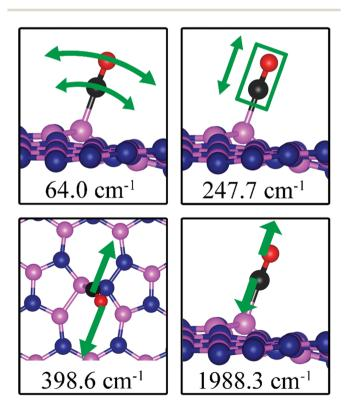
Fig. 11 Notable vibrational modes of CO adsorption on dh-BN with SW defect. The magenta, blue, black and red balls represent the B, N, C, and O atoms, respectively. Arrows indicate vibrational patterns. The rectangular encloses the atoms that concertedly move.
