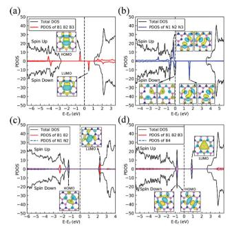
Fig. 2 Spin-polarized projected density of states (PDOS) of dh-BN with defects: (a)  $V_N$ , (b)  $V_B$ , (c) SW, and (d)  $B_N$ . The inset displays the wave function of the defect states with isosurface value of 0.001 |e|  $Å^{-1}$
