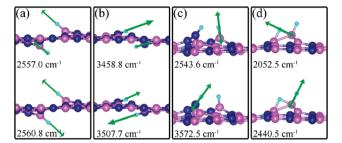
Fig. 6 Notable displacement patterns of two hydrogen atoms adsorbed on dh-BN with (a)  $V_N$ , (b)  $V_B$ , (c) SW, and (d)  $B_N$  defect. The magenta, blue, black and light blue balls represent the B, N, and H atoms, respectively. Arrows indicate displacement directions
