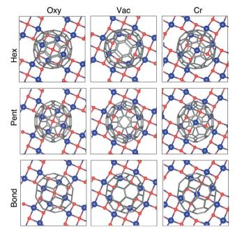
Fig. 1 Top view of the relaxed geometries of the explored configurations depending on adsorption site and relative orientation between C<sub>60</sub> and  $Cr_4O_5$ . The colour code is as follows: Cr - blue, O - red and C - grey. The Fe substrate layers are not shown.
