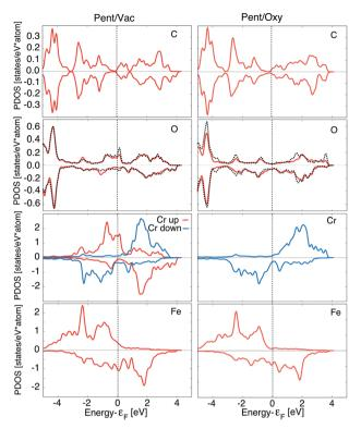
Fig. 4 PDOS on Fe and Cr (d component), O and C atoms facing to the surface (p component) for the Pent/Vac (left) and Pent/Oxy (right) configurations. Two representative Cr atoms with opposite polarization are reported for the AFM configuration. For O we report as a red line the PDOS averaged over the cell, and as a black dashed line that averaged on the four nearest neighbours to C<sub>60</sub> in the Pent/Vac configuration, and that of the O below C<sub>60</sub> for the Pent/Oxy case.
