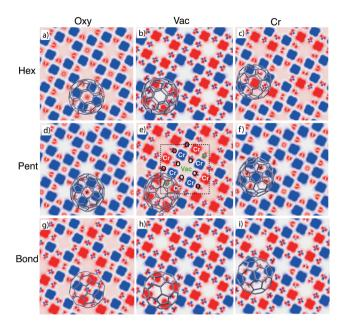
Fig. 3 Spin polarization  $\rho_{\rm up}$ - $\rho_{\rm down}$  for each pattern (top view). A cut on the surface plane passing through the Cr atoms is reported with an isosurface value of 0.02  ${\rm \AA}^{-3}$ . Red and blue areas correspond to positive and negative values of spin polarization, respectively.
