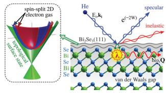
Fig. 10 HAS from topological insulator surfaces such as Bi<sub>2</sub>Se<sub>3</sub>(111) provides a sensitive probe to determine the surface phonon dispersion and energy dissipation processes in terms of the electron-phonon coupling constant  $\lambda$ . The inset on the left illustrates the surface electronic structure of Bi<sub>2</sub>Se<sub>2</sub>(111) with the Dirac cone in green and a spin-split electron gas.
