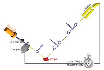
Fig. 3 Diagram illustrating the principle in a helium time-of-flight (TOF) experiment. An incident helium pulse is visible at the left-hand side of the sample, with the initial velocity distribution indicated as a single blue peak. After scattering off the surface the helium beam has excited and annihilated phonons at the surface, leading to an energy loss and an energy gain respectively, visible as two additional peaks before and after the elastically scattered fraction in the middle
