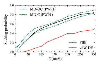
Fig. 2 Sticking probabilities for  $H_2 + W(110)$  as a function of the collision energy. Comparison between molecular dynamic classical and guasiclassical calculations (using a PES obtained with the PW91 xc-functional) from ref. 7 and our classical AIMD calculations using the PBE and vdW-DF xc-functionals.
