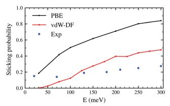
Fig. 3 Sticking probabilities for  $H_2$  + W(110) as a function of the collision energy. Comparison between initial sticking probabilities obtained in molecular beam experiments as reported in ref. 2 and classical *ab initio* molecular dynamics using the PBE and vdW-DF xc-functionals.
