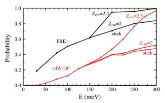
Fig. 5 Probability to reach the distance  $Z_{cm} = 2.5$  Å and  $Z_{cm} = 2$  Å for  $H_2$  molecules approaching the W(110) surface as a function of the initial kinetic energy. Black lines correspond to the use of the PBE xc-functional while red lines are obtained using the vdW-DF functional. The sticking curves from Fig. 2 and 3 are shown here as well to facilitate the comparison.
