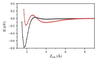
Fig. 6 Interaction energy between the W(110) surface and the H<sub>2</sub> molecule for two trajectories leading to dissociative adsorption with initial collision energy of 200 meV. The energy is plotted as a function of the vertical distance  $Z_{cm}$  between the molecule center of mass and the W surface. Both trajectories (one simulated by means of the PBE xc-functional and the other by means of the vdW-DF xc-functional) have the same set of initial coordinates.
