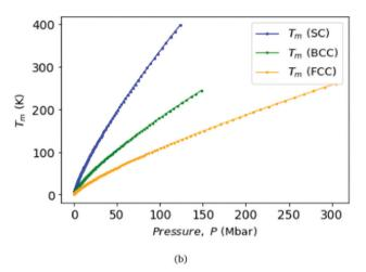
Fig. 9 We plot the Debye temperatures  $\Theta$  (top panel) and melting points  $T_{\rm m}$  (bottom panel) of MH in SC, BCC, and FCC lattice structure with the correlation with respect to the pressure, P.
