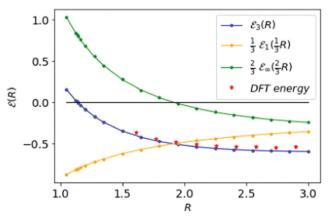
Fig. 5 The orange and green curves describe the results from D = 1 and  $D \rightarrow \infty$  respectively. The blue curve energy  $\mathscr{E}_3(R)$  represented the interpolation result at D = 3 for MH, in the SC lattice. The red points represent the results obtained from density functional theory in ref. 31. The black line shows the zero-energy line, where the blue curve goes through on R = 1.14 at a phase transition.
