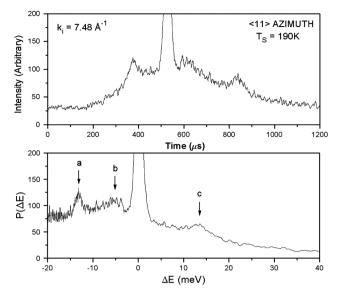
Fig. 6 Time of flight spectrum of the 52% Nb KTN target at a surface temperature of 190 K in the (11) azimuth taken at an incident angle of 42°. The upper panel shows the arrival time spectrum. The lower panel shows the transform of the upper panel into an energy transfer spectrum. The peaks a, b, and c are at energies -13.5, -5.0, 14.0 meV respectively.
