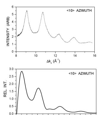
Fig. 2 Upper panel: Intensity of the He specular diffraction peak ( $\Delta K = 0$ ) in the  $\langle 10 \rangle$  azimuth as a function of the z component of the incident He atom wave vector ( $\Delta k_z$ ). The surface temperature is 190 K. Lower panel: Fourier transform of the upper panel, plotted as a function of step heights of surface terraces. The large initial peak is an artifact resulting from the limited range of experimental  $\Delta k_z$  values that go into the Fourier transform.
