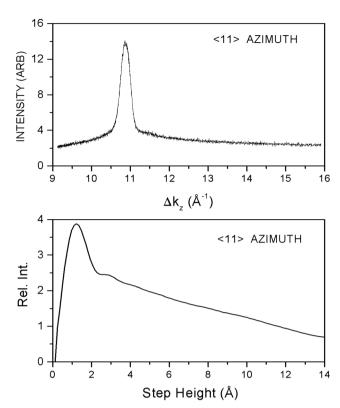
Fig. 3 Upper panel: Intensity of the He specular diffraction peak ( $\Delta K = 0$ ) in the  $\langle 11 \rangle$  azimuth as a function of the z component of the incident He atom wave vector ( $\Delta k_z$ ). The surface temperature is 190 K. Lower panel: Fourier transform of the upper panel, plotted as a function of step heights of surface terraces
