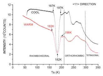
Fig. 5 Surface temperature scan of the 52% Nb KTN target in the (11) azimuth. The scans were carried out as in Fig. 4 with upper cooling curve from  $\sim\!350$  K to  $\sim\!60$  K and lower warming curve from  $\sim\!50$  K to  $\sim\!350$  K. The initial He atom wave vector  $k_i = 7.48 \text{ Å}^{-1}$ . The dotted vertical lines indicate the bulk phase transitions.
