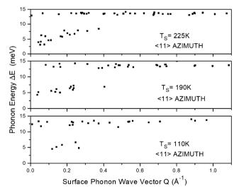
Fig. 7 Dispersion results (surface phonon energy  $\Delta E$  vs. surface phonon wave vector Q) for 52% Nb KTN in the  $\langle 11 \rangle$  azimuth at 110 K, 190 K, and 225 K. The measured  $\Delta K$  values have been folded into the first surface Brillouin zone to get Q by adding or subtracting appropriate multiples of the lattice spacing in this azimuth (2.22  $\text{Å}^{-1}$ ) (Q = 0 to 1.11  $\text{Å}^{-1}$ ).
