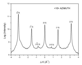
Fig. 1 Angular distribution for a 52% Nb KTN target in the (10) azimuth. The intensities are plotted logarithmically to emphasize the presence of half order diffraction peaks. The surface temperature is 190 K.
