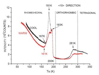
Fig. 4 Surface temperature scan of the 52% Nb KTN target in the (10) azimuth. The specular He scattering intensity yielded the upper curve as the target was cooled from  $\sim$  350 K to  $\sim$  80 K and the lower curve as it was warmed from  $\sim 60$  K to  $\sim 325$  K. The He atom wave vector  $k_i = 7.88 \text{ Å}^{-1}$ . The dotted vertical lines indicate the bulk phase transitions.
