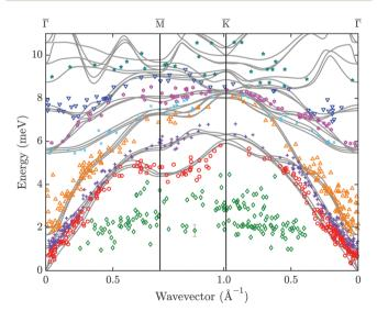
Fig. 3 Experimental surface phonon dispersion of  $Sb_2Te_3(111)$  from helium atom scattering (symbols) in comparison with DFPT calculations for three quintuple layers in the lower part of the phonon spectrum (solid grey lines).<sup>30</sup> The assignment of the data points (colour and tag) to different modes is based on the proximity to the theoretical modes. One exemplary error bar is shown at an energy of  $\approx 2$  meV.
