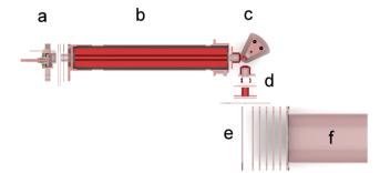
Fig. 1 Schematic of the apparatus SurfTOF with the major parts labelled; (a) electron impact ion source, (b) quadrupole mass filter, (c) heated target surface, (d) ion optics and second electron impact ion source, (e) orthogonal extraction region of a reflectron TOF-MS, (f) drift tube of the TOF-MS
