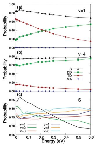
Fig. 3 Quasi-classical  $O_2(v, J = 1)$  reaction probabilities on Cu/Ru(0001)as a function of the incidence energy, for a surface temperature  $T_{\rm s}$  = 350 K. (a) Vibrational state v = 1; (b) v = 4; (c) total sticking probabilities for vibrational states v = 1 to v = 6. S stands for total sticking probability, DD for direct dissociation, TD for trapping dissociation, and MA for molecular adsorption
