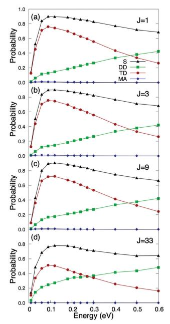
Fig. 2 Quasi-classical  $O_2(v = 0, J)$  reaction probabilities on Cu/Ru(0001) as a function of the incidence energy, for a surface temperature  $T_s = 350$  K. (a) J = 1; (b) J = 3; (c) J = 9; (d) J = 33. S stands for total sticking probability, DD for direct dissociation, TD for trapping dissociation, and MA for molecular adsorption.
