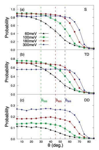
Fig. 4 Quasi-classical  $O_2(J = 0, v = 0)$  reaction probabilities on  $Cu_{1ML}/I$ Ru(0001) as a function of the initial polar angle, for  $T_s = 350$  K. (a) Total sticking; (b) trapping dissociation; (c) direct dissociation. The dashed lines mark the  $\theta_{tes}$  values, i.e. the maximum incidence polar angle for which the reaction probability does not depend on  $\theta_i$ .
