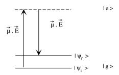
Fig. 2 The ground and the first excited electronic states are represented by  $|g\rangle$  and  $|e\rangle$ , respectively. The wave function for the initial and final vibrational state (for Stokes shift) in the ground electronic state is represented by  $|\psi_i\rangle$  and  $|\psi_f\rangle$ , respectively
