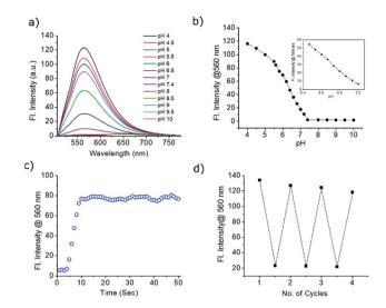
Fig. 2 (a) Fluorescence response of the probe PS-OH ( $20~\mu M$ ) in PBS buffer at different pH ranging from 4 to 10. (b) Changes in the fluorescence maximum at 560 nm at different pH. Inset: linear variation of fluorescence intensity with pH between 5.6 and 7.2. (c) Response time of PS-OH upon addition of TFA ( $20~\mu L$ ). (d) Reversibility in the fluorescence switching of the probe PS-OH between pH 4 and 7.4.
