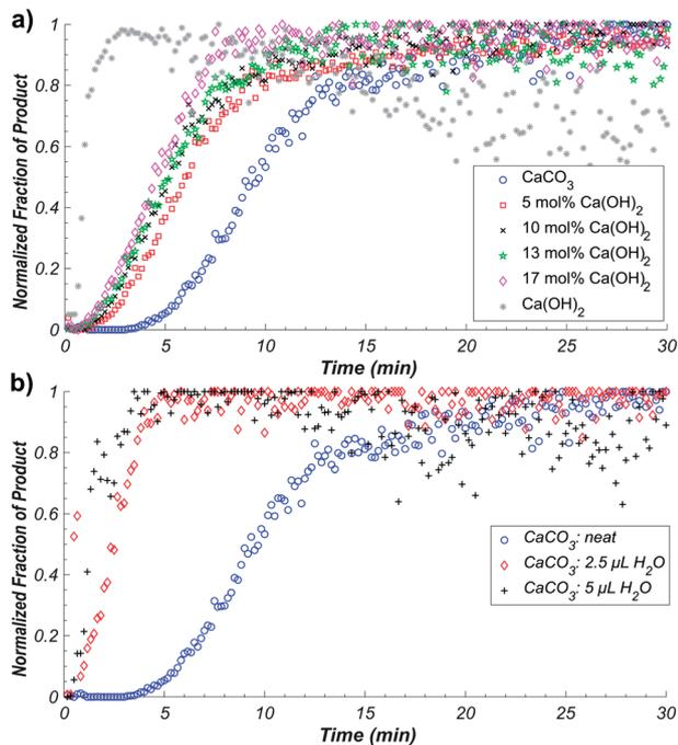
Fig. 4 (a) Monitoring the relative rates of formation of **1** from  $\text{CaCO}_3$  (blue) and  $\text{Ca(OH)}_2$  (grey), as well as various mixtures. (b) The addition of small volumes of water to the synthesis of **1** from  $\text{CaCO}_3$ , results in a significant increase in reaction rate as observed by *in situ* Raman spectroscopy. In each case the total weight of solid reactants was approximately 180 mg.
