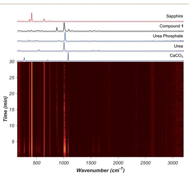
Fig. 2 (Bottom) *In situ* Raman spectra of the neat milling reaction between  $\text{CaCO}_3$ , urea, and urea phosphate. Brighter colour denotes higher intensity. (Top) Raman spectra of reactants (blue), the product (black), and background from the sapphire milling jar (red) with individual spectra of reactants and product above the 2D plot.
