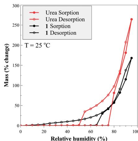
Fig. 6 Adsorption/desorption branches of RH on urea and **1**.
