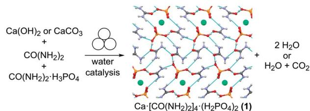
Fig. 1 Mechanochemical synthesis of the agrochemical cocrystal **1** from urea, urea phosphate and either calcium hydroxide or carbonate. Calcium ions are shown in green, and hydrogen bonding interactions are displayed in light blue for **1** (CSD code URECAP10).
