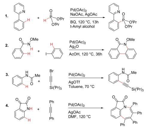
Scheme 1 Palladium acetate catalyzed reactions involving C-H activation and reductive elimination in the presence of various silver salt additives.<sup>24</sup>
