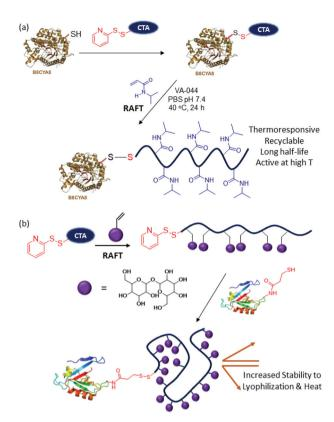
Fig. 4 (a) 'Graft-from' strategy for the synthesis of the thermoresponsive enzyme-polymer conjugate, <sup>82</sup> and (b) 'graft-to' strategy for the synthesis of the trehalose based protein–polymer conjugate for protein stabilization. <sup>83</sup> Adapted from De, Datta *et al.* <sup>82</sup> with permission. Copyright © 2018 by American Chemical Society. Adapted from Maynard *et al.* <sup>83</sup> with permission. Copyright © 2012 by American Chemical Society.
