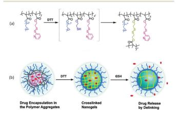
**Fig. 10** (a) Synthetic approach, and (b) crosslinking strategy of PDS bearing polymers to fabricate a redox-responsive nanogel based drug delivery system. <sup>124</sup> Adapted from Thayumanavan *et al.* <sup>124</sup> with permission. Copyright © 2010 by American Chemical Society.
