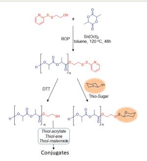
**Fig. 5** Synthesis of thiol-reactive PDS-containing biodegradable polymers.  $^{87}$  Adapted from Ghosh *et al.*  $^{87}$  with permission. Copyright © 2012 by American Chemical Society.
