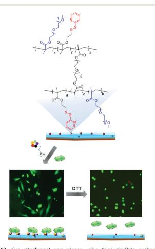
**Fig. 12** Cell attachment and release using thiol-disulfide exchange reaction on a hydrogel interface. <sup>137</sup> Adapted from Sanyal *et al.* <sup>137</sup> Copyright © 2018, American Chemical Society.
