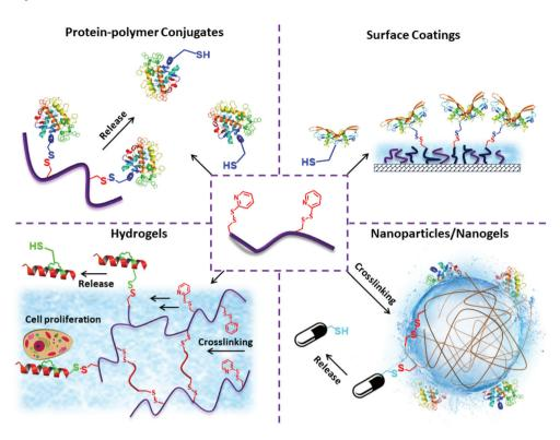
Scheme 1 Schematic representation of common applications of the PDS functional group based exchange chemistry in fabrication and functionalization of polymeric materials.
