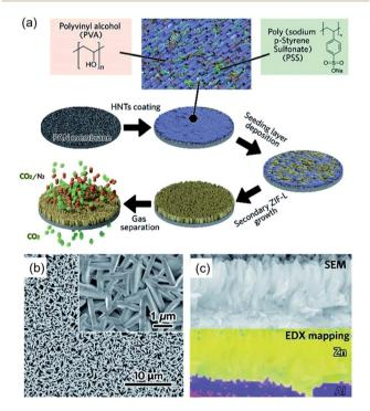
Fig. 5 (a) Schematic illustration for the preparation of the PAN-HNTs-ZIF-L membrane. (b) SEM image of the top-surface of the PAN-HNTs-ZIF-L membrane, and (c) EDS mapping and reference SEM image of the PAN-HNTs-ZIF-L membrane cross-sectional region. Reproduced with permission.84 Copyright@2019 The Royal Society of Chemistry.
