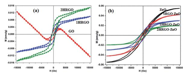
Fig. 14 *M-H* curves of (a) GO, 1HRGO and 2HRGO, and (b) ZnO, SRGO–ZnO, 1HRGO–ZnO and 2HRGO–ZnO nanocomposites, reproduced with permission from ref. 90, copyright 2018, Springer.
