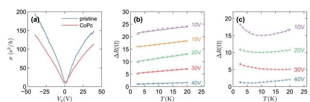
Fig. 19 (a) Conductivity versus gate voltage plots for pristine graphene/h-BN (blue line) and CoPc decorated graphene/h-BN (red line). Temperature dependence of resistivity at different gate voltages for (b) pristine graphene/h-BN, and (c) CoPc decorated graphene/h-BN, reproduced with permission from ref. 155, copyright 2018, Elsevier.
