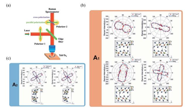
Fig. 8 (a) Schematic of the angle-resolved polarized Raman spectroscopy of TaIrTe $_4$  samples. Raman intensities of (b)  $A_1$  and (c)  $A_2$  modes as a function of the sample rotation angle and the corresponding phonon modes in the atomic view. The scattered dots are the experimental data and the solid lines are the fitting curves. Reproduced from ref. 49 with permission from Wiley-VCH.
