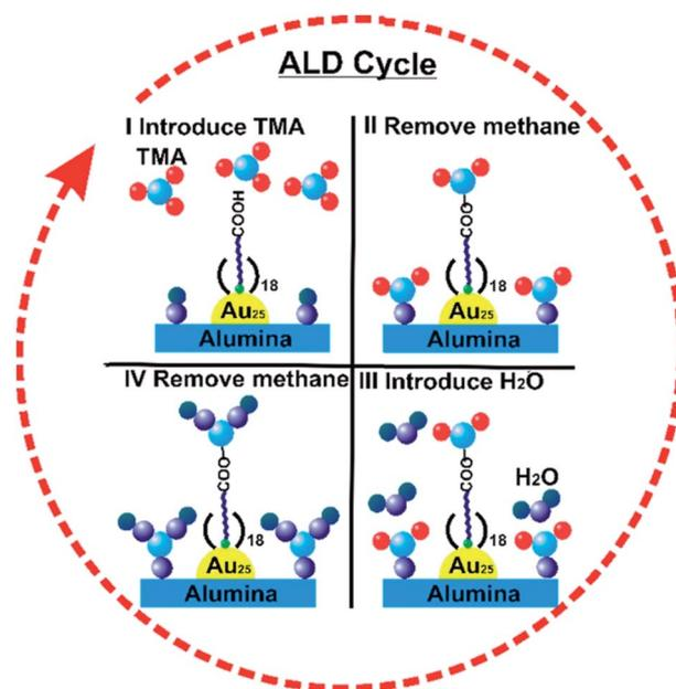
Fig. 11 General scheme of alumina deposition over  $\text{Au}_{25}(\text{MUA})_{18}/\text{Al}_2\text{O}_3$  by atomic layer deposition. Reprinted with permission from ref. 111. Copyright 2018 American Chemical Society.
