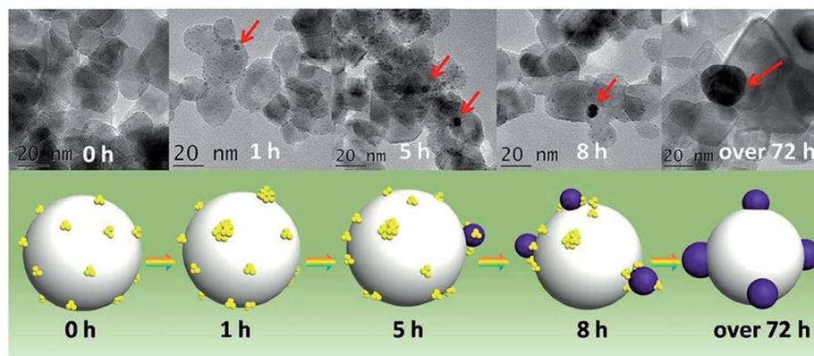
Fig. 8 Illustration of the *in situ* transformation of Au clusters into Au nanoparticles on nanoporous titania nanotube arrays. Reprinted with permission from ref. 93.
