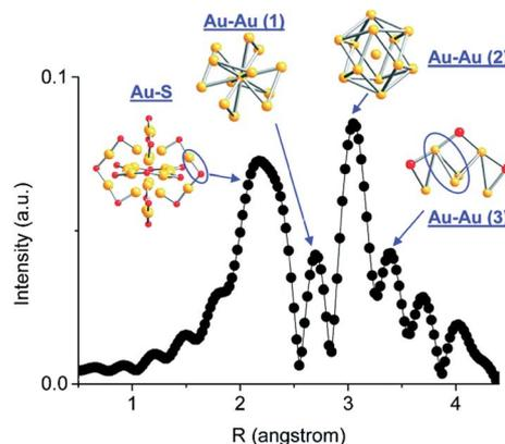
Fig. 2 Simulated FT-EXAFS of  $\text{Au}_{25}(\text{SR})_{18}$  clusters. The simulation was done by averaging the EXAFS from all representative Au sites of  $\text{Au}_{25}$  ( $k$ : 3–14.5 Å<sup>-1</sup>,  $k^1$  weighted). The spectrum was phase-corrected using the Au–S peak. Reprinted with permission from ref. 43. Copyright 2011, American Chemical Society.
