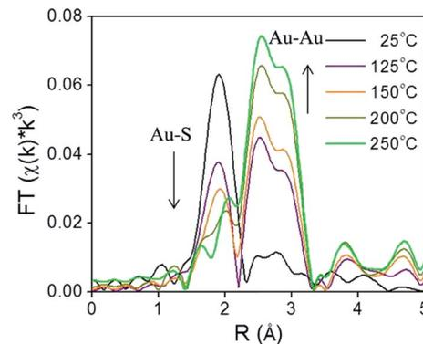
Fig. 4 Au L<sub>3</sub> edge EXAFS spectra in the R space of Au<sub>25</sub>(SR)<sub>18</sub> clusters on carbon (with no phase shift correction). Reprinted with permission from ref. 54. Copyright 2013, American Chemical Society.
