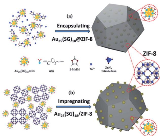
Fig. 10 Illustration of  $\text{Au}_{25}(\text{SR})_{18}$  clusters (a) encapsulated in, and (b) impregnated onto, a ZIF-8 metal–organic framework. Reproduced with permission from ref. 110. Copyright 2018 John Wiley and Sons.
