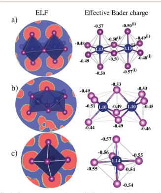
Fig. 4 Electron localization function (ELF) and effective Bader charge (e) of inorganic  $\operatorname{Bi}_{x}\operatorname{I}_{y}^{\delta-}$  moieties of perovskites (a) **1**, (b) **2** and (c) **3**. Along bismuth-iodide planes, the colors blue and red in the ELF plots represent electron charge depletion and accumulation, respectively
