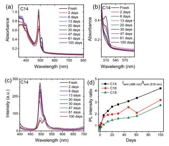
Fig. 3 (a) and (b) Absorption and (c) photoluminescence spectra of thin films of  $(C_{14}H_{29}NH_3)_2Pbl_4$  2D perovskite thin films stored under ambient conditions. (d) Variation in the photoluminescence intensity ratio of shorter wavelength peak (496 nm) to the longer wavelength peak (516 nm).
