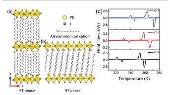
Fig. 1 Schematic of the crystal structure of the (C<sub>14</sub>H<sub>29</sub>NH<sub>3</sub>)<sub>2</sub>Pbl<sub>4</sub> perovskite (a) at room temperature (RT) and (b) at high temperature (HT) with interdigitated arrangement of alkylammonium chains. (c) Differential scanning calorimetry (DSC) curves of the  $(C_nH_{2n+1}NH_3)_2PbI_4$  (n = 14, 16 and 18) 2D perovskite powder samples measured in both heating and cooling cycle.
