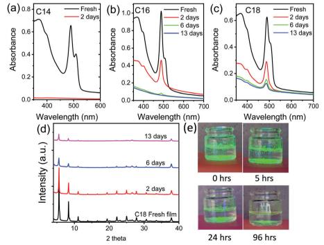
Fig. 4 Absorption spectra of (a)  $(C_{14}H_{29}NH_3)_2PbI_4$ , (b)  $(C_{16}H_{33}NH_3)_2PbI_4$  and (c)  $(C_{18}H_{37}NH_3)_2PbI_4$  2D perovskites thin films immersed in water. (d) XRD pattern of  $(C_{18}H_{37}NH_3)_2PbI_4$  thin film immersed in water and (e) bright green light emission from the  $(C_{14}H_{29}NH_3)_2PbI_4$  powder sample immersed in water and kept under continuous UV light (365 nm) illumination.
