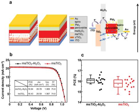
Fig. 1 (a) Schematics of device configurations of the PSCs based on mesoporous TiO<sub>2</sub>/Al<sub>2</sub>O<sub>3</sub> and mesoporous TiO<sub>2</sub> scaffolds, together with the band diagram of the PSC based on the mesoporous TiO<sub>2</sub>/Al<sub>2</sub>O<sub>3</sub> scaffold. (b) Current density-voltage curves of the best cells in their respective counterparts. The inset shows the photovoltaic parameters. (c) PCE distributions of the PSCs based on different mesoporous scaffolds.
