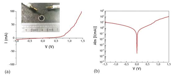
Fig. 6 (a) I–V dark measurment of Al/VACNTs/ZnO/perovskite/spiro-OMeTAD/EGa:In device – 0.0079 cm<sup>2</sup> active area and (b) semi-logarithmic representation.
