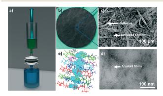
Fig. 1 (a) Schematic diagram of syringe-aided filtration setup. (b) Cropped filter membrane. (c) SEM image of the membrane surface. (d) Transmission electron microscope image of the amyloid fibrils. (e) Schematic representation of the putative binding of radionuclides on to the amyloid fibrils surface.
